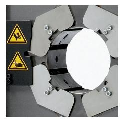
Parker's TH8-380 production crimper is designed to withstand the rigors of high volume production hose assembly manufacturing. The electronic controls come preloaded with Parker hose part numbers and crimp specifications to make hose selection quick and easy.
